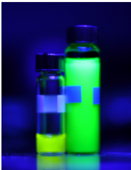
FIG. 6. (Color online) Photograph of CdTe quantum dot (left) and \text{LaF}_3:\text{Ce}/\text{CdTe} nanocomposite (right) aqueous solutions under a UV lamp.
